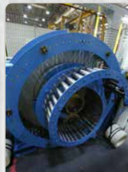
Nonstop Production thanks to Strip Accumulation
